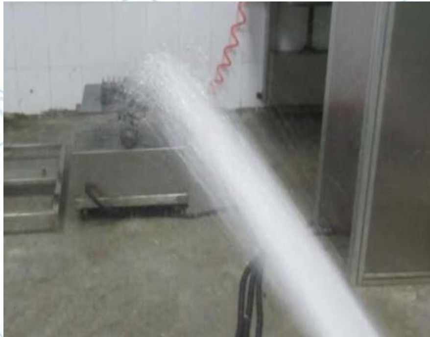
Photo 4: Test result after IP6X and IPX6 test
