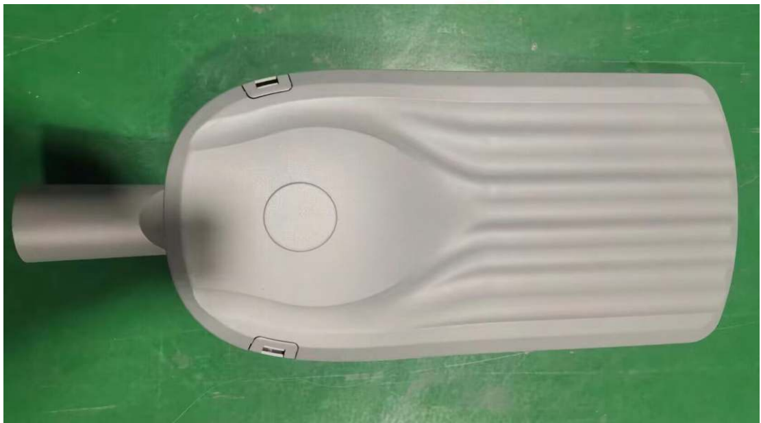
Photo 4: Test result after IP6X and IPX6 test
