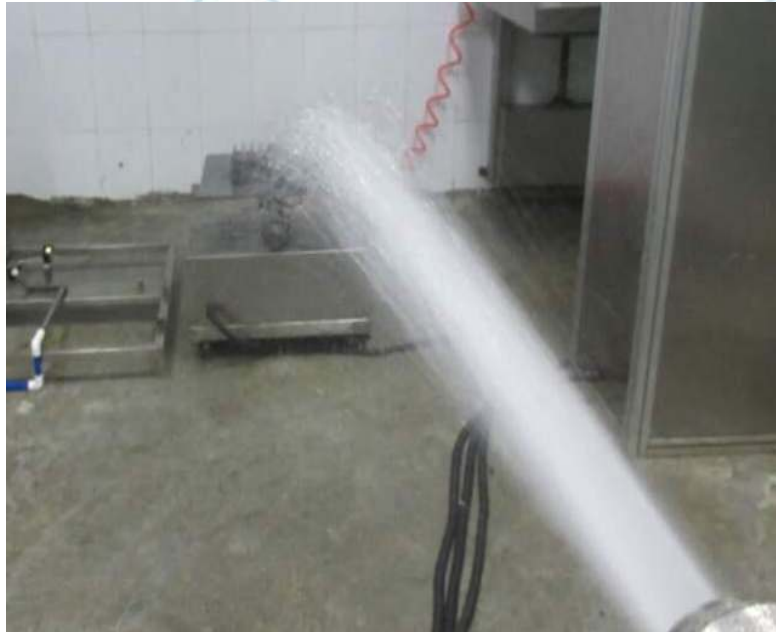
Photo 3: IPX6 test of model LM-AP-200W
