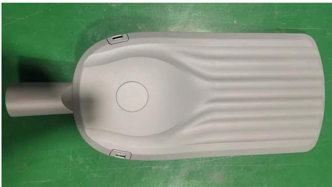
Photo 4: Test result after IP6X and IPX6 test
