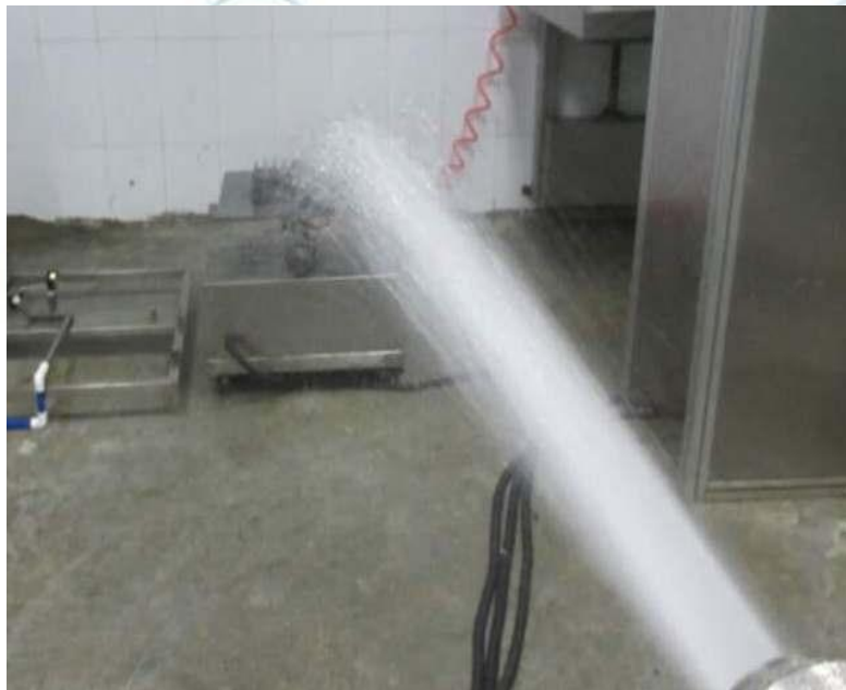
Photo 3: IPX6 test of model LM-AP-200W
