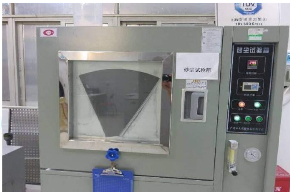
Photo 2: IP6X test of model LM-AP-200W
